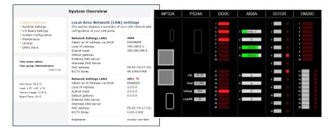
**Easy access to setup/data** The RTU32M web Server allows access to the RTU setup. Change port settings, update firmware, monitor network activity and more from a web interface. Publish user displays as html pages for display on your tablet or phone.
