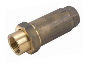
Dual Check Valves are utilised for protection from cross contamination of non potable water with potable water. They are used in low hazard conditions such as rain water tank systems and domestic meter connections.
