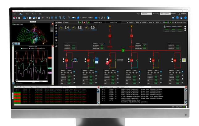
SurvalentONE SCADA can be configured to provide operators with relevant information at a glance. Maps, single line diagrams, schematics, event summaries & alarms are shown in the SmartVU application.
